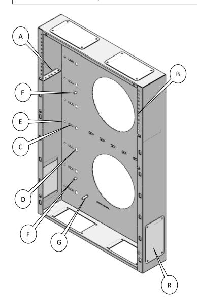
The MiniRaQ<sup>™</sup> System can be mounted on a variety of vertical substrates including wooden framing studs 16" on center (C), solid or block concrete walls, and approved plywood used for NEC panel mounting.
